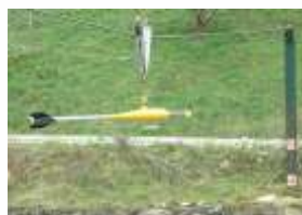
Universal current meter in use
