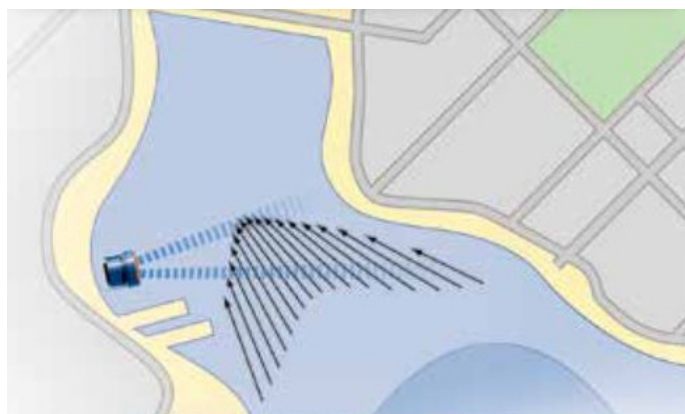
The ChannelMaster H-ADCP is installed on a riverbank or near-shore structure to acquire real-time velocity, stage, and discharge data.
