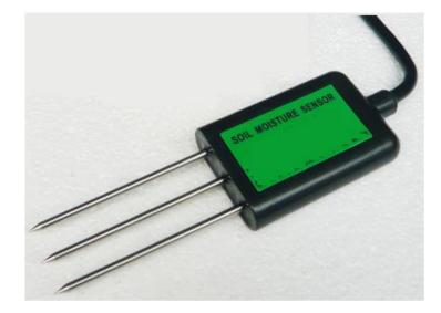
This Soil Moisture sensor is a FDR (frequency domain reflectometry) based sensor that is used to measure Soil volumetric water content (VWC) and temperature. The sensor consists of highly corrosion resistant electrodes. This sensor is designed to be used for portable as well permanent installations placed in the soil.
