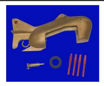
These are medium-weight suspended-sediment samplers for hand line or sounding reel suspension. The DH-59 sampler comprises a streamlined bronze casting, 15 inches (38 cm) long, which partially encloses a pint-size (0.47-liter) sample container (sold separately). This sampler weighs approximately 22 pounds (10 kg), and is equipped with a tail vane assembly to orient the intake nozzle of the sampler into the approaching flow as the sampler enters the water.
