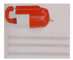
This sampler is used in shallow streams when the product of the depth (in feet) and velocity (in feet/sec) does not exceed approx. 10. This sampler is used with wadding rod suspension.
