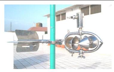
"Virtual" make Vertical Axis-Cup Type Water Current Meter is used to measure Velocity of water flow directly in m/s. The spindle carrying the cup wheel freely rotates in the pivot assembly. The magnet and reed switch assembly produces one pulse per rotation. The rotation of the Water Current Meter is sensed by sensor & gives pulsed output signal.
