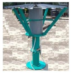
This is a Alter style snow gauge as per IS 6806-1973 for use with a precipitation gauge to improve the catch of the snow. Snow is an important component of the hydrological cycle in mountainous and polar areas, and also in mid-latitude countries. The Important parameters for hydrological purposes are snow depth, density and snow water equivalent. This Snow gauge is used to measure Snow Water Equivalent. This System comes with one Snow Gauge, one sample collection bottle and one measuring Jar.
