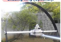
Shading Ring is used for diffuse radiation measurement. Need to adjust thrice in a day. It is an optional Item and Sold at Extra Prices.
