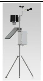
"Virtual" make Automatic Weather Station is a fully computerized, digital and self contained power source system, fitted with Data Logger and battery charging solar panel with rechargeable, maintenance free batteries complete with sensors mounted on a tripod stand with sealed waterproof IP65 enclosure for Data Logger, Solar charger and battery.
